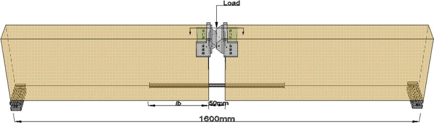
Fig. 1: Pullout-bending test set-up
