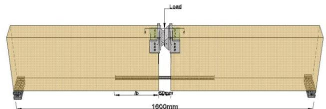
Figure 2: Pull-Bending Test Set-up
