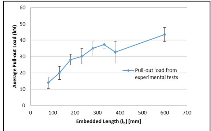
Figure 5: Average Failure Load vs Embedded Length
