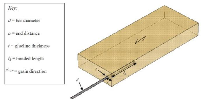
Figure 1: Specimen Geometric Variables
