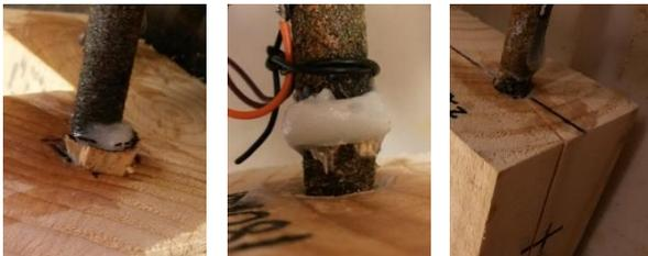
Figure 4: Failure modes observed: a) Shear in timber; b) Rod/Adhesive Failure; c) Timber Splitting
