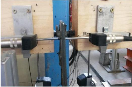
Figure 3: Transducer Set-up Used to Monitor Movement
