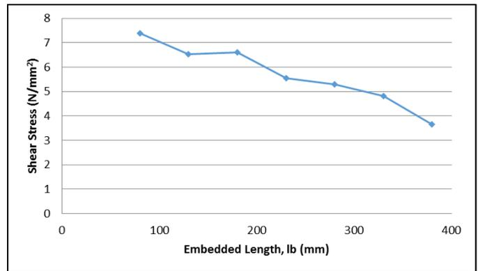
Figure 6: Peak Shear Stress at Timber/Adhesive Interface
