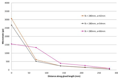
**Figure 6.** Stress distribution along glued length with increasing edge distance at a load of 10kN
