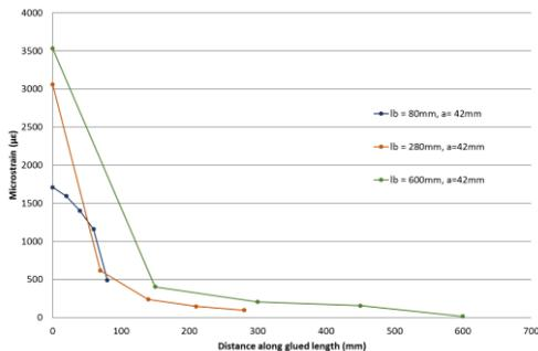
**Figure 7.** Stress distribution along the glued length with increasing embedded length at a load of 10kN
