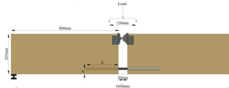
Figure 1. Pull-bending test set-up
