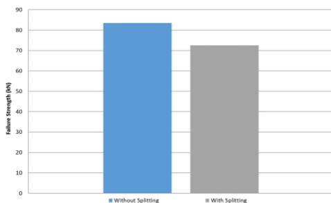
**Figure 3.** Comparison of failure strength of specimens with and without splitting
