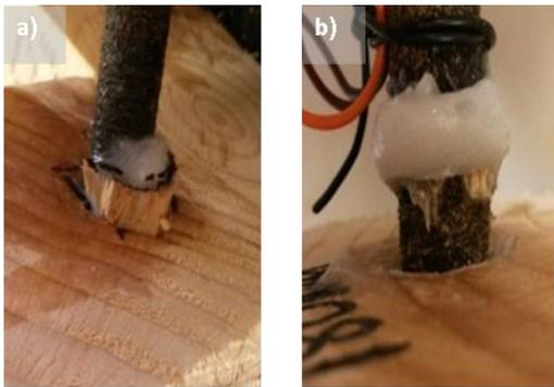
**Figure 2.** Failure modes observed a) shear in timber, b) rod/adhesive failure
