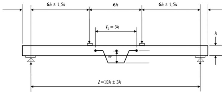
Fig. 3 Beam bending set-up (EN 408, [2])
