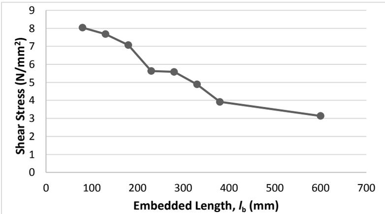
Figure 5: Peak Shear Stress at Timber/Adhesive Interface
