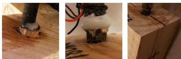
Figure 3: Failure modes observed: a) Shear in timber; b) Rod/Adhesive Failure; c) Timber Splitting
