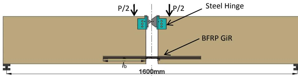
Figure 1: Pull-Bending Test Set-up
