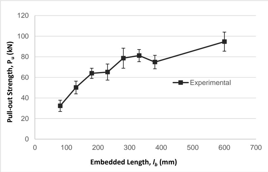
Figure 4: Pull-out strength with increasing Embedded Length
