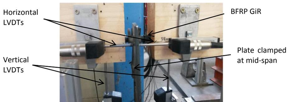
Figure 2: LVDT Set-up
