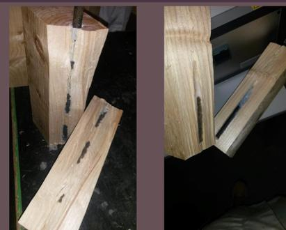
Figure 7: Delamination
