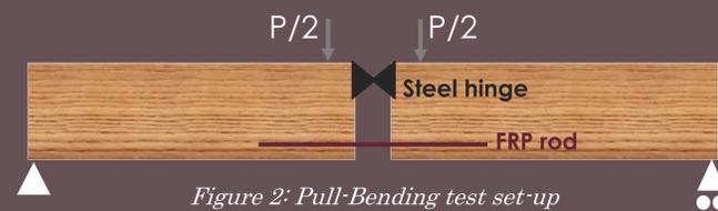
Figure 2: Pull-Bending test set-up
