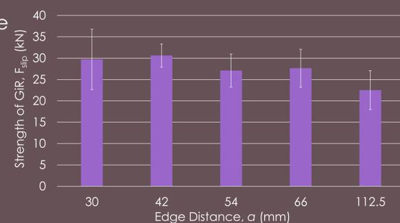
Figure 4: Pull-out force at Slip limit
