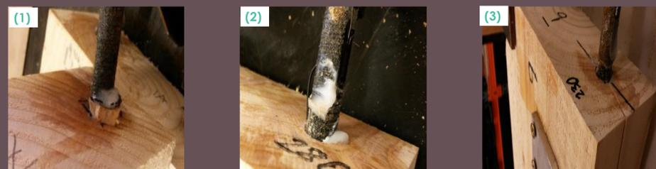
Figure 5: Failure modes : (1) Shear plug, (2) Rod/adhesive failure, (3) Splitting
