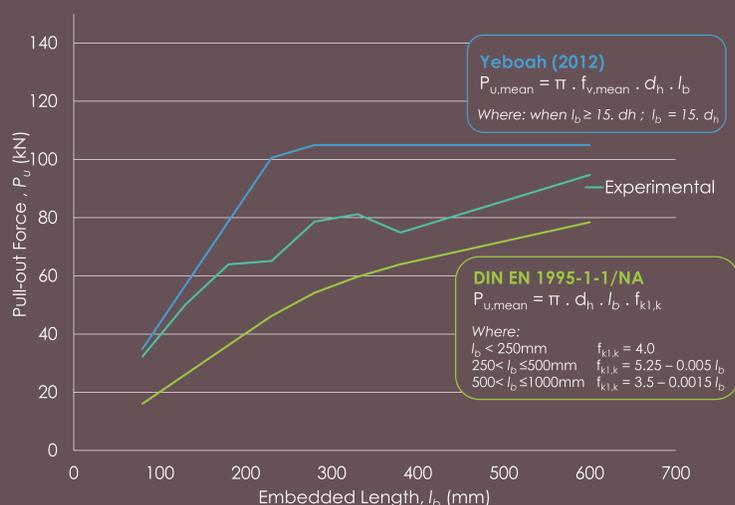
Figure 3: Pull-out capacity with increasing embedded length
