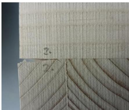
Figure 9. Delamination of specimen 2. after vacuum-pressure cycle
