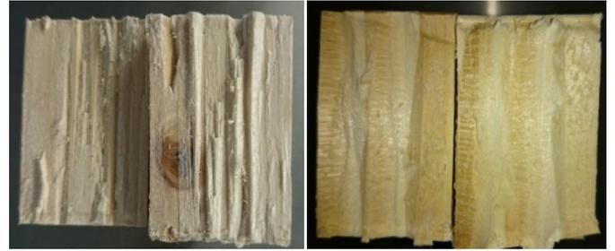
Figure 7. Glue line 7a (left, 75% wood failure) and 8c (right, 100% wood failure) after test
