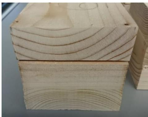
Figure 8. Delamination of specimen 6. after vacuum-pressure cycle
