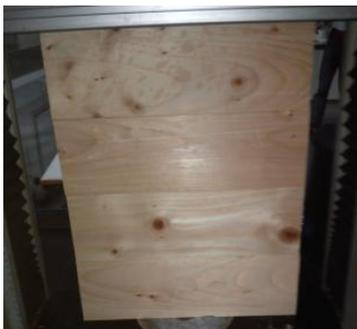
Figure 1. Pressing of the shear test specimens
