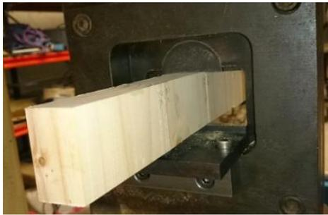
Figure 5. Test bar during testing in shearing tool
