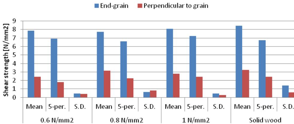
*Figure 3. Shear strength values*
