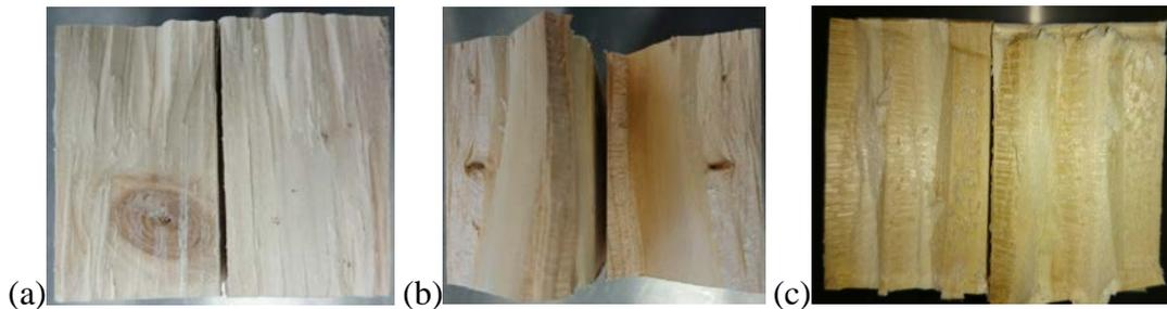
Figure 4. Glue lines with 60% wood failure loaded perpendicular to grain (a), 100% wood failure loaded perpendicular to grain (b), and 100% wood failure loaded at end-grain (c)
